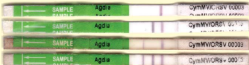
Step 5 Read the strips. A = CyMV indicator line; B = ORSV indicator line; C = control line.
